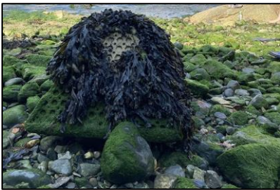
A small, trial eco-block, 20 months after being deployed
