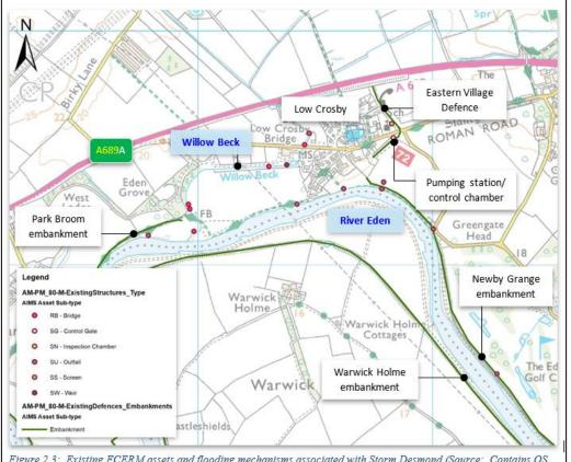
Figure 2.3: Existing FCERM assets and flooding mechanisms associated with Storm Desmond (Source: Contains OS data © Crown copyright and database right (2021). Derived from Environment Agency Asset Information Management System (AIMS) data (2016).
