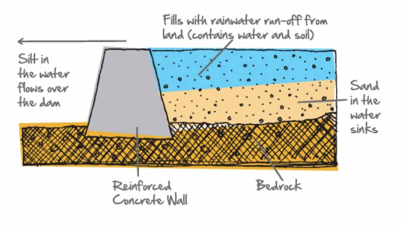
1-3% of water flowing downstream is retained behind the wall
