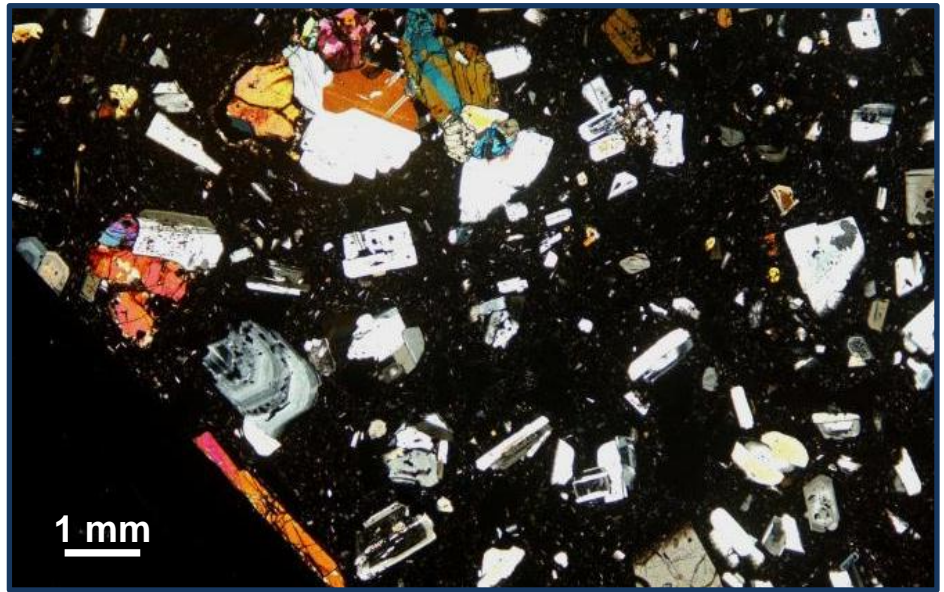
Above: Light microscope image; the brightly coloured crystals are pyroxene. Left: electron microscope image of a plagioclase phenocryst (mid-grey); the light grey crystals are apatite (page 33), and the bright white crystals are titanomagnetite (see below). Below: the jagged edge of a calcium-rich pyroxene, showing it has started to break down. Right: Iron-rich streaks in a pyroxene phenocryst.
